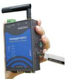
**Step 2:** After removing the cover, insert the SD memory card as shown.
